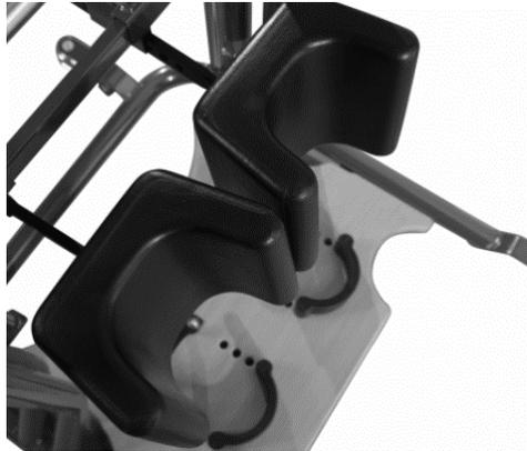
*Figure 6: Adjustment of the knee pads*
