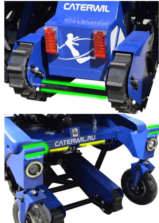
Fig. 2.1. Handles for transport
