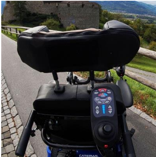
Fig. 9.3. Additional remote control for the attendant
