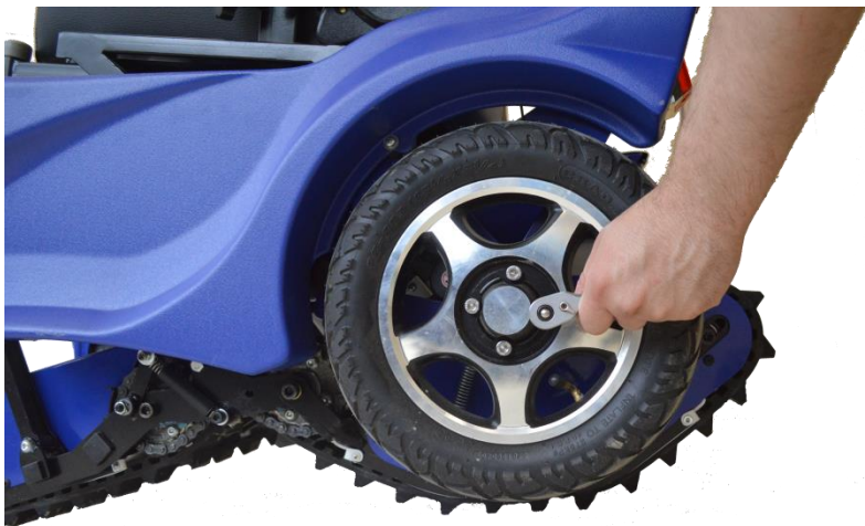
Fig. 12.1. Tightening the drive wheel screws
