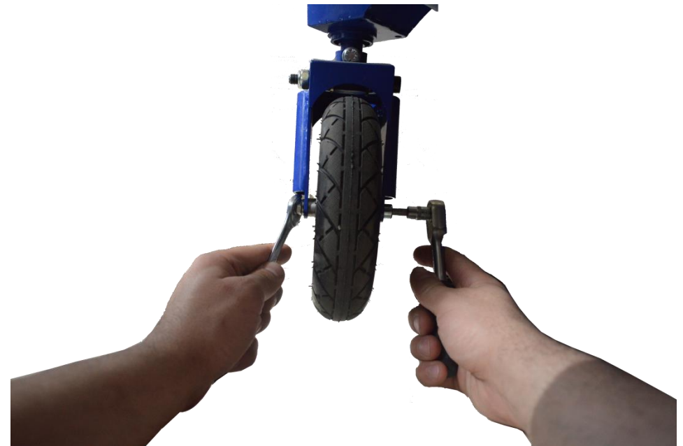
Fig. 12.2. Tightening the driven wheel axle
