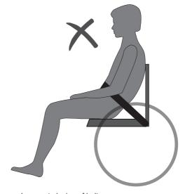
Incorrect placing of belt
