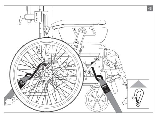
Cirrus G5 has marked off four points that must be used when securing the wheelchair.
