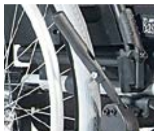
// BRS060010 Brake lever extension, knee-lever brake, fold-down
