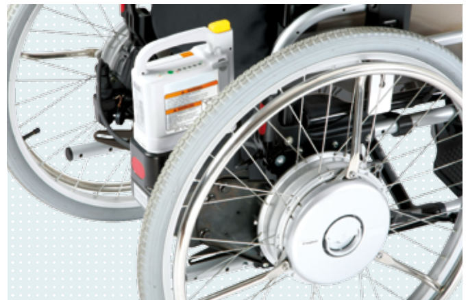
• e-support add-on drive (servo auxiliary drive operated via the push rings)
