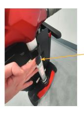
7. Pull on the catch (arrowed left) on the tiller to unlock. Then pull up the tiller until it is set at the correct height for the user. Push the catch to lock the tiller.
