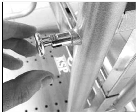
d. Release it so that it remains in the extended position and then repeat this operation for the both locking mechanisms
