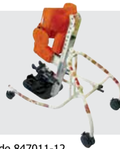
Code 847011-12 Robin - full options configuration, with abductor complete with postural unit for the pelvis, frame adjustable of 30° by a mechanical system, supports for knees and trunk adjustable in height, footrest adjustable in height
