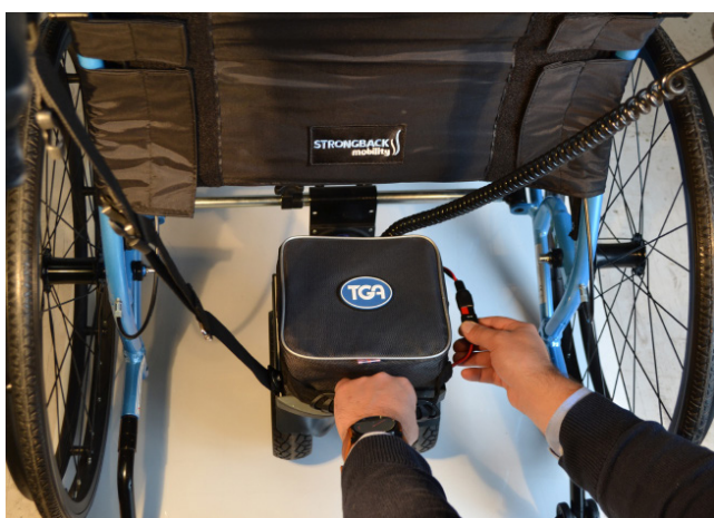
Fig 4 Fitting and connecting battery
