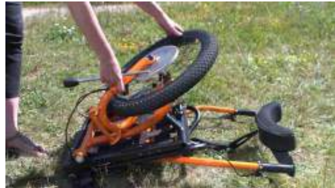
2- Remove the pin and security pin from their place and rotate the wheel
