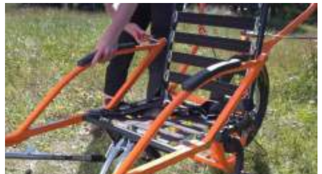
12- Do the same for the seat and tighten the screws. Proceed the same way on the second arm.
