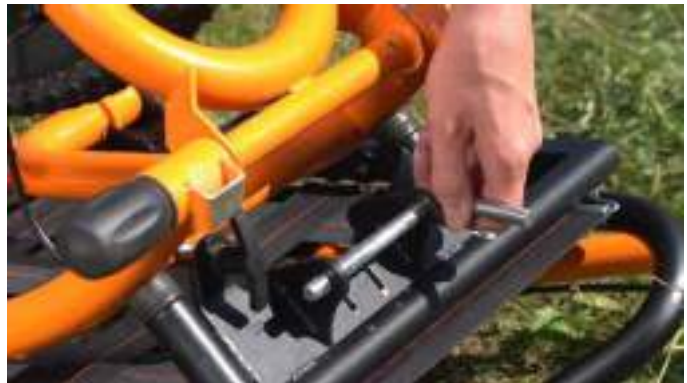
4- Remove the security pin and pull the axle out of its compartment
